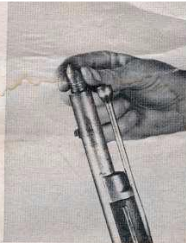
3 Inserting bullet. Again note position of fingers and hand
