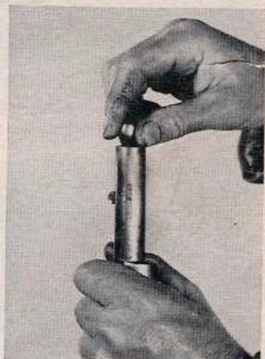
7 Springing the rammer. First be sure that the cap or primer is removed. Tap the small end of the rod on the face of the breech screw. If the rifle is not loaded, the rod will have a metallic ring. A dull thud will indicate a lead bullet is still in the bore. Do not use the cup end of the ramrod. After a period of firing, the bore will be slightly fouled and this fouling will cause the head to stick and the ramrod will be quite hard to withdraw
